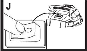
Plug in the vacuum and turn it on using the switch on the vacuum as illustrated in section (J)
