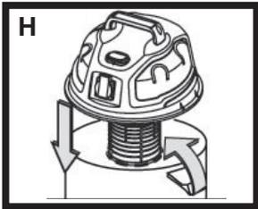
Put the top of the vacuum back in place and lock it using the latches on each side of the vacuum as illustrated in section (H)
