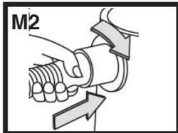
Insert the hose in the suction port and turn it clock wise until you hear a click to lock the hose in place as illustrated in image M2
