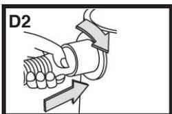
Insert the hose in the suction port and turn it clock wise until you hear a click to lock the hose in place as illustrated in image D2
