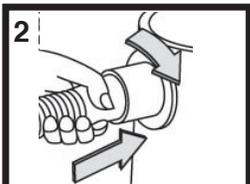
Insert the hose in the suction or blower port and turn it clock wise until you hear a click to lock the hose in place as illustrated in image 2
