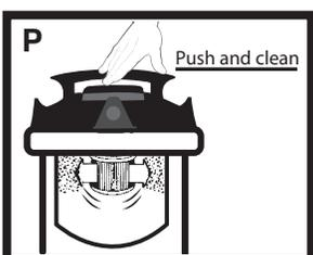
Step 2: Block the suction port as illustrated in section (O) and press the shake button for 1 second, then release. Repeat this process a minimum of 10 times.
