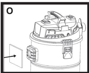
Step 1: Block the suction port as illustrated in section (O)
