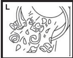
Make sure the debris container is empty before using the blower function, otherwise debris will blow out which may be harmful and cause severe injuries or death.
