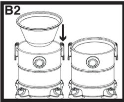
If using dust collector, install it laying flat on the edge of the vacuum as illustrated in section (B2)
