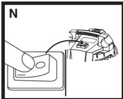
Turn on the vacuum using the switch as illustrated in section (N)
