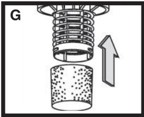
To install the foam filter, simply slide it on the filter cage as illustrated in section (G)
