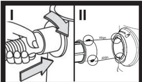
Align the pins on the hose with the gap on the suction or blower port of the vacuum as illustrated in image II.
