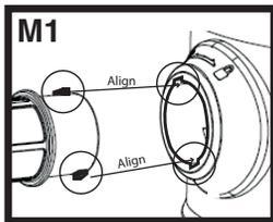
Align the pins on the hose with the gap on the blower port of the vacuum as illustrated in image M1.
